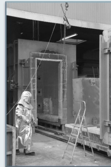
Oven for testing the fire-resistant properties of products
