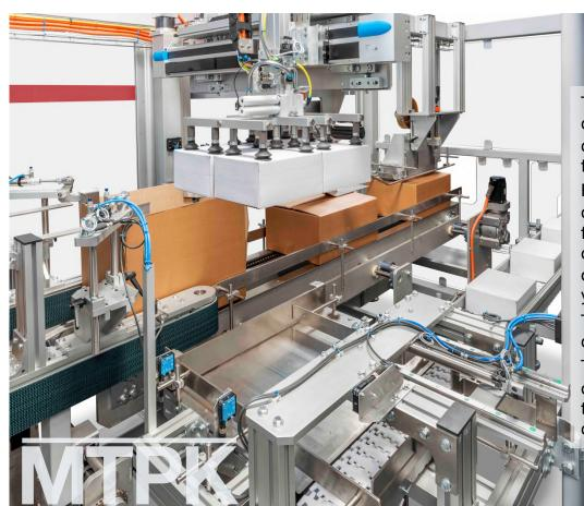
The MTPK integrated top loader case packers are designed for the automatic erection, filling and closing, by tape or hot melt, of RSC/HSC/OSC fluted cardboard outer cases.
