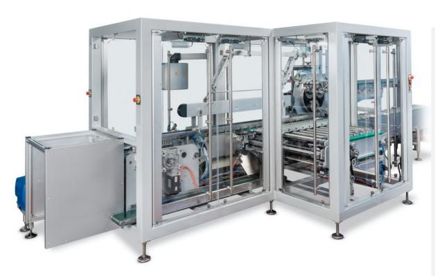
The HML series of intermittent (i) and continuous (c) horizontal cartoners represents the state of the art in mid to high speed requirements boxing applications.
