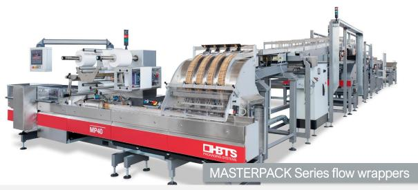
HBTS designs and manufactures a variety of pillow pack style flow wrappers suitable to serve low, mid and high end speed requirements.
