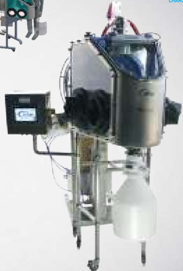
DRUM IRIS REACTOR CHARGING
