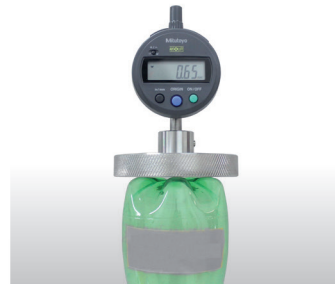
BASE CLEARANCE CHECK
