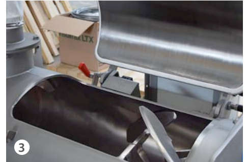
Loading and inspection hatch with safety block
