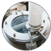
Closure plug, with viewing glass and filter sleeve
