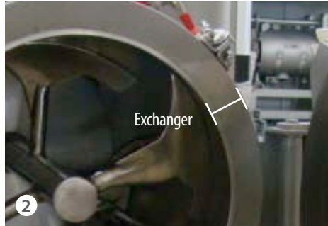
2 Mixing chamber complete with heat exchanger on the cylindrical part (optional)
