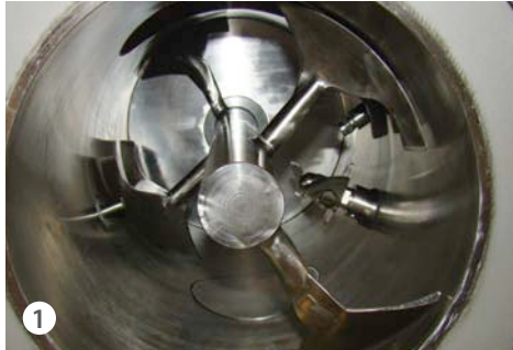
1 Internal chamber with welded ploughs, and polishing treatment
