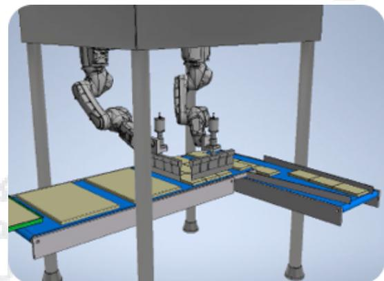
Both robotic and non-robotic applications for piercing and shaping pizzas and buns, consisting of Delta robot, holding structure and transfer conveyor.
