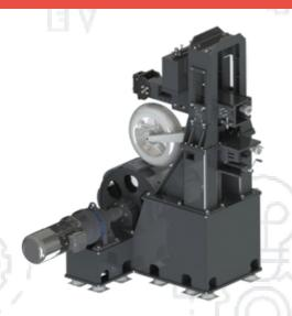
The solution consists of a cab with a **test bench** inside, through which the speed that the tyre will have to withstand on the road is reproduced.
