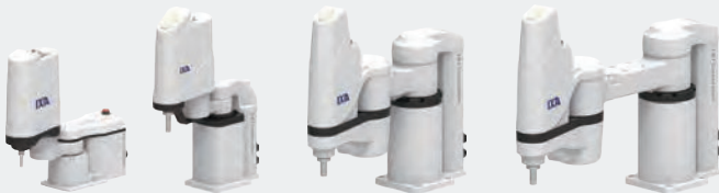
Standard and High-speed Type (Vertical axis stroke: 50/150/180/330mm)
